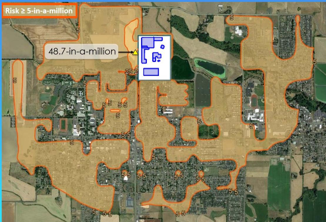
2,149 receptor points in conjunction with **terrain modeling** used to mathematically model isopleths.
